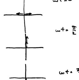
• Intensity of output light has only DC and  $2\omega$  frequency components.
