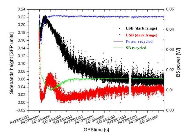
•One hour of thermal transient can be seen in the signals
