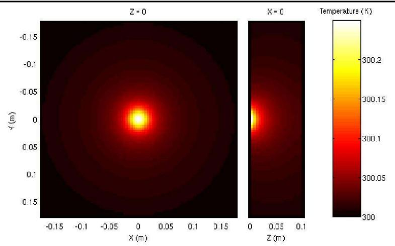
Temperature distribution after 12 hours of YAG heating
