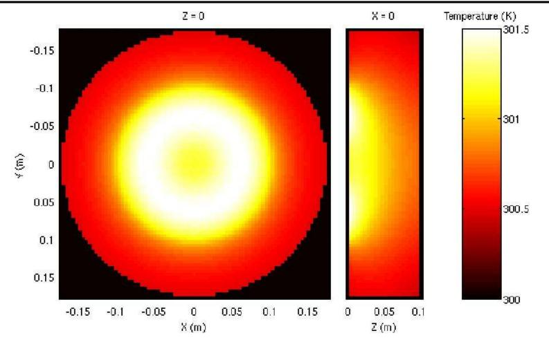
Temperature distribution after 12 hours of CO2 ring beam heating (1W)
