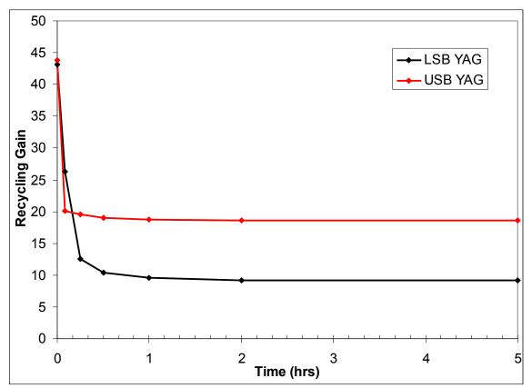
$\cdot$  Fast reduction in sidebands gain with time constant  $\sim 10$  min
