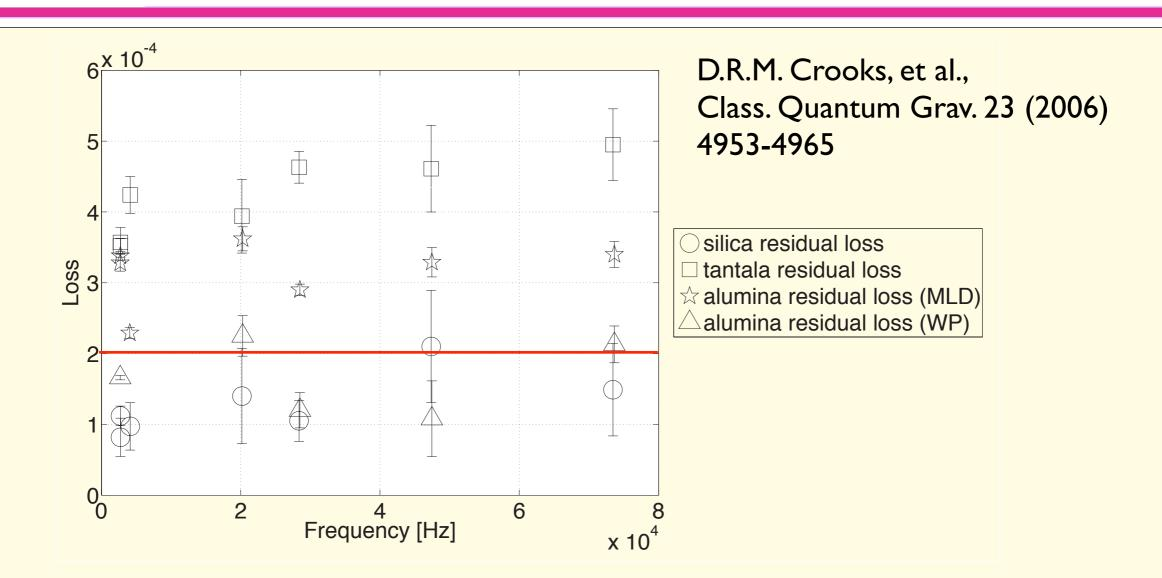
**Figure 4.** Residual losses for SiO<sub>2</sub> ( $\phi_{SiO_2}$ ), Ta<sub>2</sub>O<sub>5</sub> ( $\phi_{Ta_2O_5}$ ) and Al<sub>2</sub>O<sub>3</sub> ( $\phi_{Al_2O_3}$ ) as a function of frequency. Note that for the Al<sub>2</sub>O<sub>3</sub>, losses are quoted for both the sample obtained from MLD and that obtained from Wave Precision.
