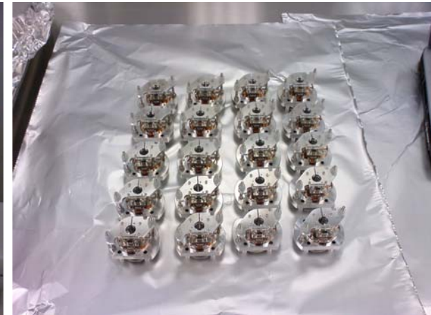
Assembled BOSEMS at testing station
