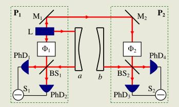
In LIGO there is resonance gain of signal, in displacement-noise-free configuration — no resonance gain.
