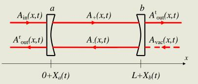
Experimenter can manipulate by linear combination of the reflection-output  $A_{out}^{r}(x, t)$  and transmission-output  $A_{out}^{t}(x, t)$  signals.
