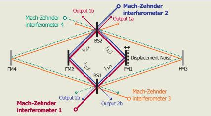
Manipulating by outputs one can exclude information on displacement of each 6 mirrors and keep information on GW signal.
