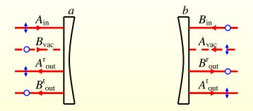
The pump wave through mirror *a* has detuning  $\delta_1$ , polarization in the plane of incidence and denote it with  $A_{in}$ ; the pump wave through mirror *b* has different detuning  $\delta_2$ , polarization orthogonal to the plane of incidence and is denoted with  $B_{in}$ . Corresponding vacuum pumps through mirrors *b* and *a* are denoted with  $A_{vac}$  and  $B_{vac}$ .
