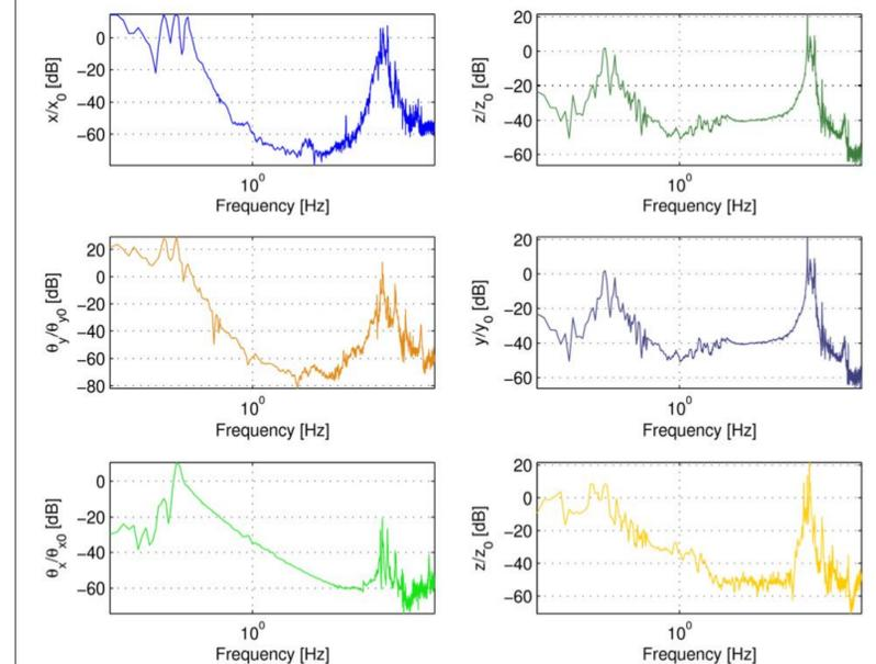
Initial transmissibilities (transfer functions between ground and isolated platform motion). The commissioning of the device was not completed.
