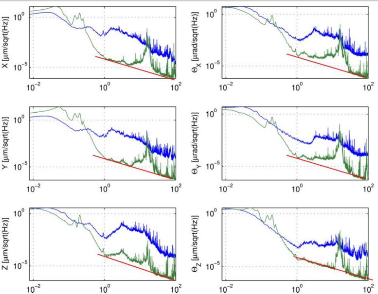
Seismic noise power spectral densities of all 6 DOFs obtained at the LIGO LASTI MIT Facility (blue-ground, green-optical table, red-geophone noise). Attenuation in the frequency range from 15Hz to 40Hz is spoiled by the spurious and still undamped pitch and roll resonances of the stabilizing device. Resonance below the Hz are the also undamped rigid body modes of SAS. The offset payload introduce coupling among the DOFs.
