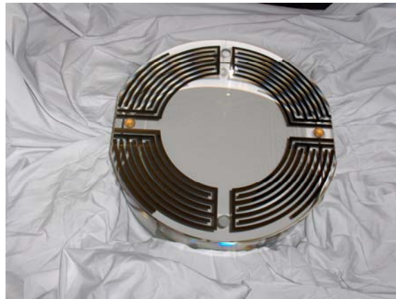
Reaction mass with 4 quadrant gold coating for electrostatic drive (ESD)
