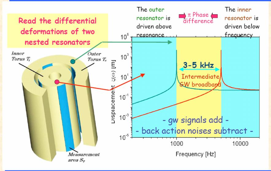
At kHz frequencies, sensitivity expected to be comparable with the interferometric detectors
