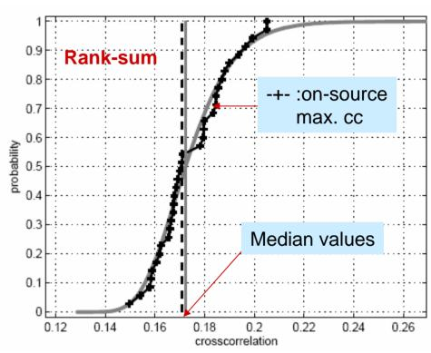
Result of tests: Null hypothesis cannot be rejected. No GW signal seen from both statistical searches.
