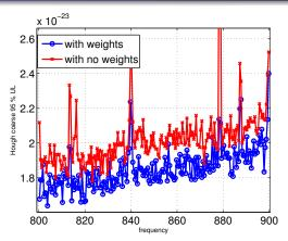
Average improvement by using weights in this band is 9.2 multi-IFO case (but only  $\sim$  6% for single IFO)
