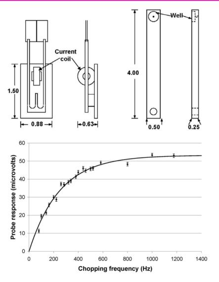
See P060053-Z, "Developing a Capacitive Probe for Measuring Surface Charge on In-Vacuum Optics".
