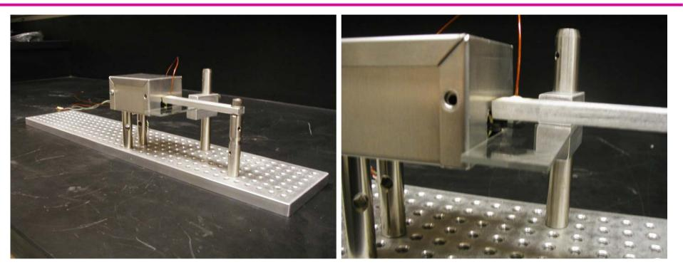
A reference cavity chamber is used for the vacuum chamber, with a turbomolecular drag pump to achieve a pressure of 10<sup>-5</sup> torr. This table can be slid in and out of the chamber by removing the end viewport.
