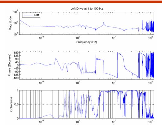
This transfer function shows the response of the top left OSEM of the local control on the main chain. The drive is at the same location.
