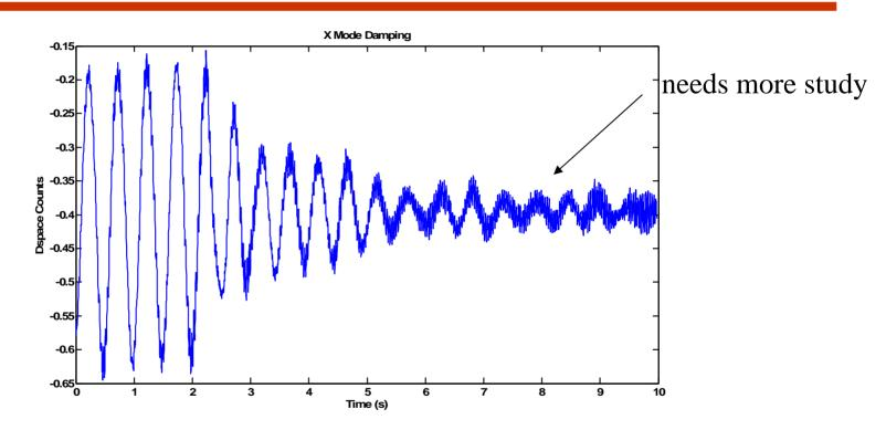
This is the response of the local control on the X Mode. The controller has a zero at DC and 2 poles at about 8 Hz. This motion was damped in about 5 seconds.
