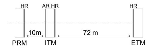
Recycling cavity unstable at low power as in LIGO 1, and AdLIGO Radii of curvature: PRM: 5.8 km, ITM: 4.0 km, ETM: 720m
