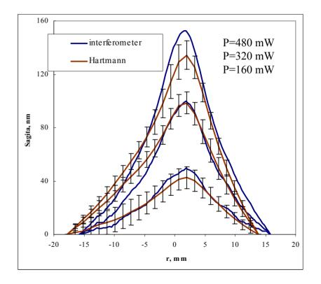
Wavefront distribution when a sample made of BK7 glass was heated by a  $CO_2$  laser beam with different power
