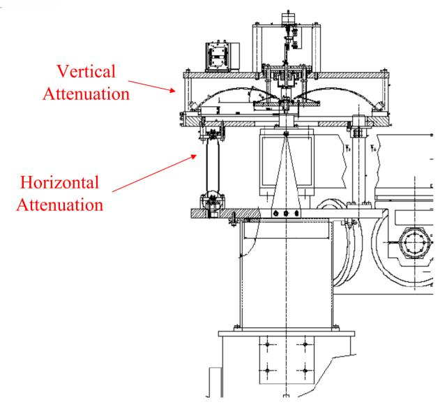
the LIGO Deep Fall Back solution prototype for on-pier pre-attenuator
