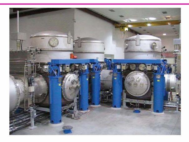
Why has LLO been 'down' for half a year? An extra active seismic isolation stage has been installed at LLO, between the piers and the external seismic support structure.
