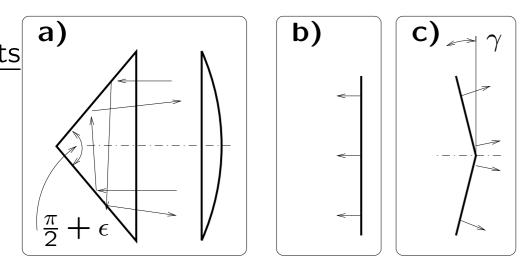
(a). Expose perturbation:  $\epsilon \neq 0$ . It produces the transformation of incident plane wave front (b) into a "broken" front of reflected wave (c) with angle  $\gamma = 2\epsilon$  for 2-hedral prism or with angle  $\gamma = 2\epsilon\sqrt{2/3}$  for 3-hedral prism (if only one plane is declined).
