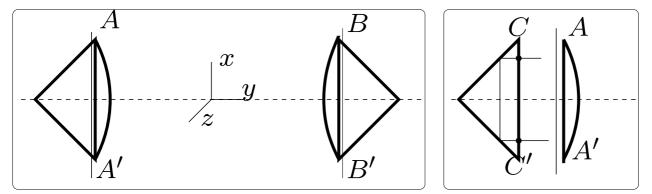
The distorsion of optical mode may be a source of additional noise in FP cavity (non elaborated problem).
