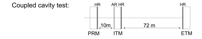
Recycling cavity unstable at low power as in LIGO 1, and AdL Radii of curvature: PRM: 5.8 km, ITM: 4.0 km, ETM: 720m
