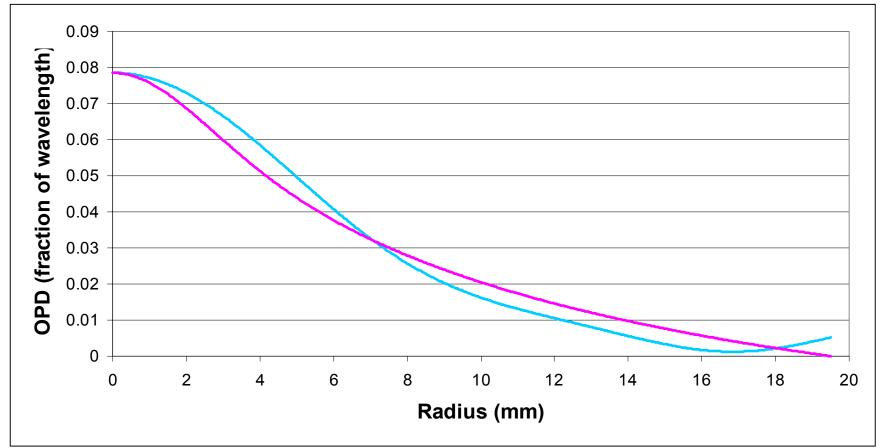
Theoretical vs Analyzed Data optical path distortion using off-axis Hartmann.
