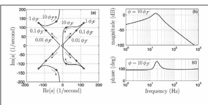
FIG. 4: Dynamical behavior of the test mass. (a) Poles of the transfer function  $\tilde{T}(\omega)$  as the cavity tuning is varied over
