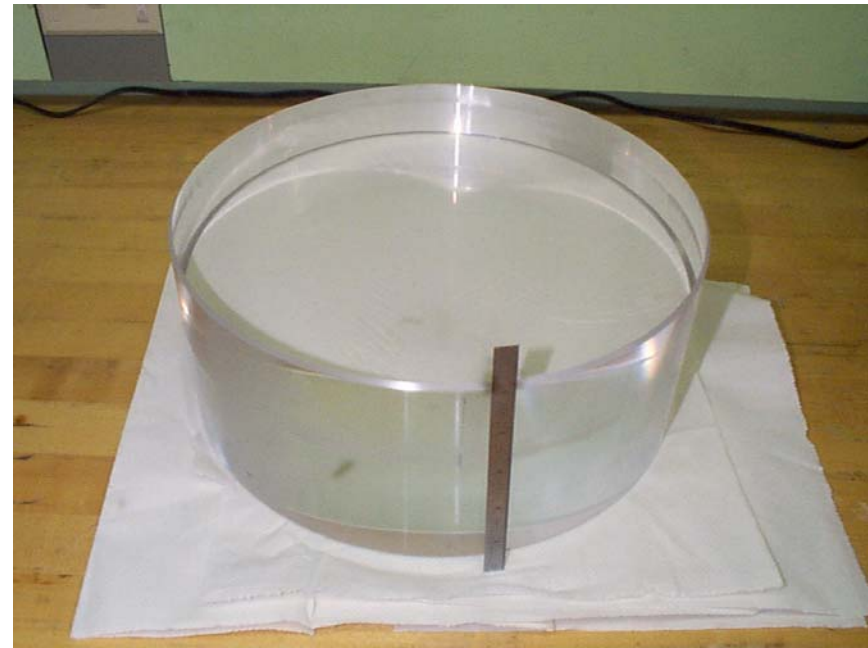
Full-size Advanced LIGO sapphire substrate
