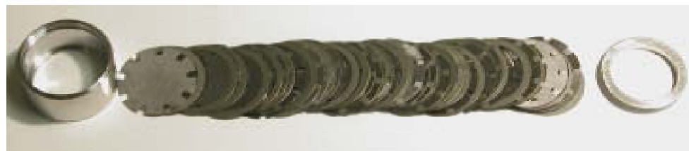
DARHT 2 distributed target for 4 pulses
