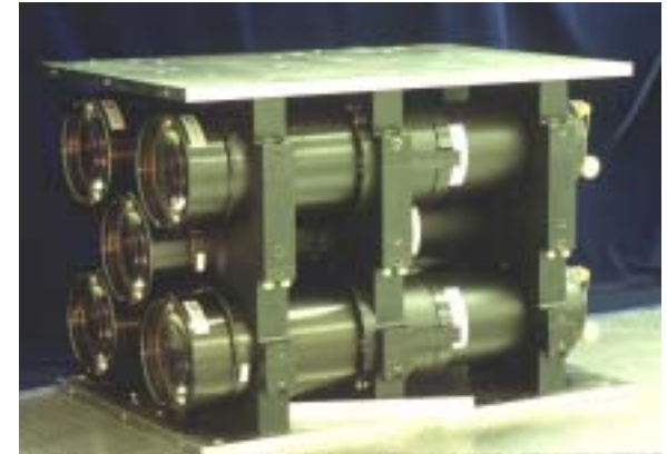
Camera array with 165-mm f1.2 lenses, <0.1% geo. distortion, 400:1 contrast ratio
