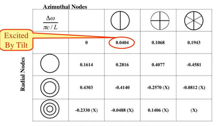
X → indicates diffraction losses per bounce > 1%
