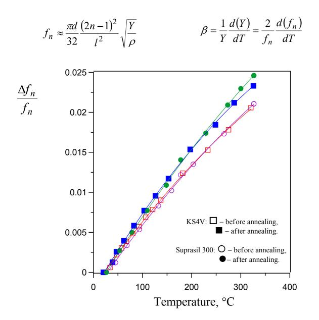
Temperature coefficient of the Young's modulus  $\beta$  in fibers with  $d \approx 250 \ \mu m$
