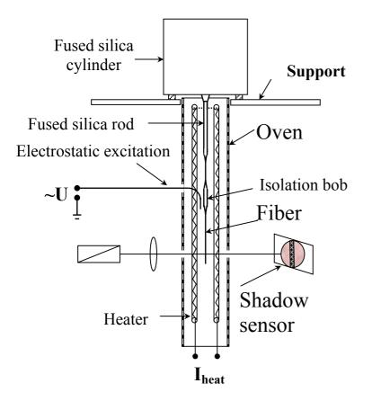
**Fiber**  $l \approx 60 \text{ mm}, d \approx 250 \text{ }\mu\text{m}$
