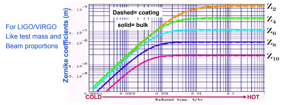
Allows fit to single beam power scaled TL distortion for unknown bulk to coating absorption ratio.
