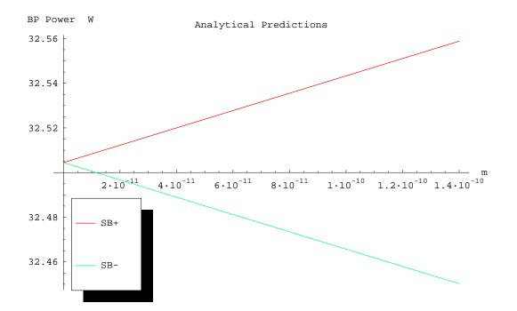
When the sidebands are not anti-resonant a slight change of the length of the two arms makes a difference in their recycling cavity power although there is no other distortion and the two Fabry-Perot cavities are completely identical.
