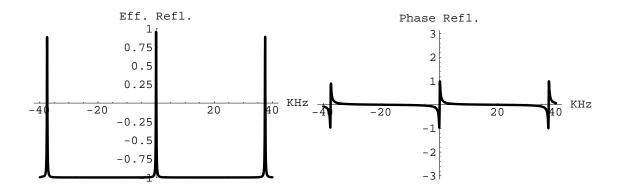
$$r_{eff}^{CR}(\delta\phi) \simeq +1 e^{i(\frac{1+r}{1-r})\delta\phi}$$
