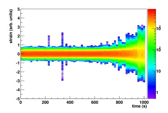
**Example of PeakMon output.** Each vertical stripe is a histogram of a 16-second frame of AS\_Q data. Three things can be seen: an occasional non-gaussian bursty segment, a gradual increase in noise due to misalignment, and (for the sharp-eyed) an overly-broad center possibly indicating a significant line feature in the data.
