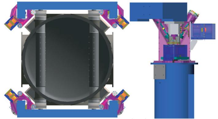
• External, mm-range, pre-isolation stage (**EPI**). Platform servoed with large gain to local sensors, corrected for coupled ground noise and global signals. Effective in 0.1–10 Hz band.
