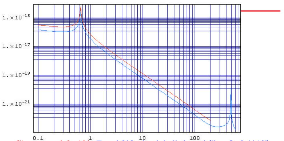
Glassy metal  $Q=10^4$ , Fused  $SiO_2^{10}$  dumb bell shaped fiber  $Q=8.4*10^8$ ,  $10*3000=30,000~\mu\text{m}^2$ , 357  $\mu\text{m}$  diameter,  $100,000~\mu\text{m}^2$ , 29 40 Kg mirror
