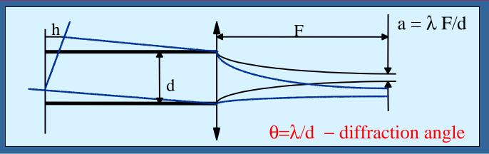
In linear electrodynamics the major limitation to measure wave front deviations angles comes from a finite size of the focal spot  $h=\lambda/20...\lambda/50$  is achieved by an accurate measurement of the transverse beam distribution
