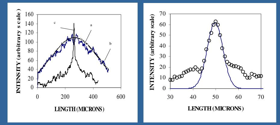
Of all the tested substances, the minimum size of a self-focusing point is in benzene, i.e. 5  $\mu$ m at the length of a nonlinear cell of 60 cm, which results in the precision of wave front inclination measurements  $\lambda/3000$ .
