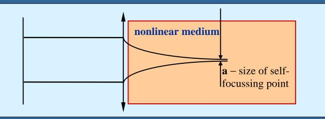
How to get  $\lambda/1000$ ? Use self-focusing to decrease the size of the focal spot. At P=P<sub>critical</sub> a  $\rightarrow 0$  and is determined by nonlinear medium properties
