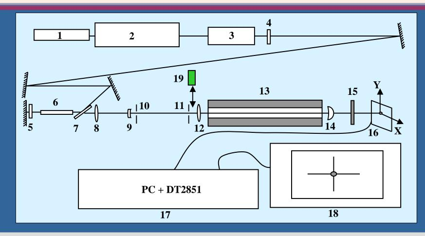
1 – HeNe laser; 2 – Nd master oscillator; 3 – single pulse selector;  $4 - \lambda/2$ ;
