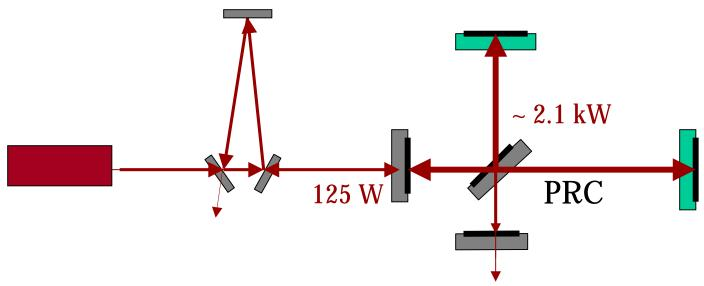
Sapphire optics, rear coated, r ~ 0.9975, thermal correction Fused silica optics, PRM thermal correction?
