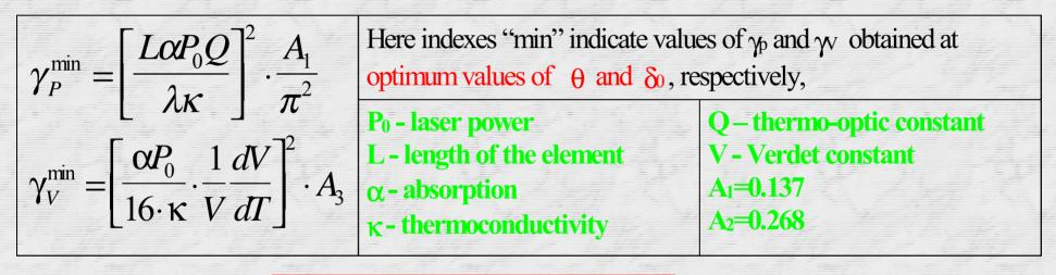
$$\frac{\gamma_V^{\min}}{\gamma_P^{\min}} = 2 \cdot \left[ \frac{\pi}{16} \cdot \frac{\frac{1}{V} \frac{dV}{dT}}{Q} \cdot \frac{\lambda}{L} \right]^2 \le 0.01$$
