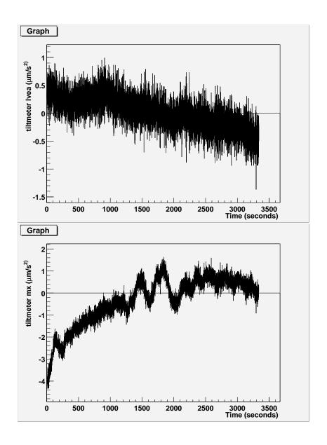
The long term drifts seen in station MX are possibly due to thermal effects (e.g. differential expansion of the tiltmeter legs, this is under investigation).
