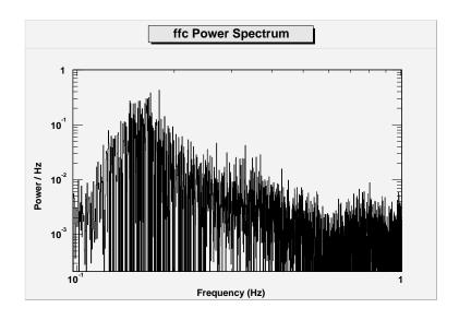
Power of error signal corrected with the tiltmeters:
