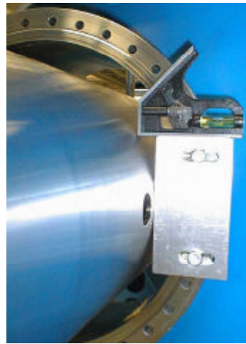
Figure 29. Support Tube Centering Block
