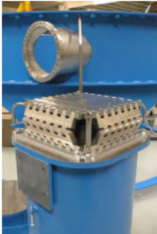
Figure 8. Scissors Table Installed
