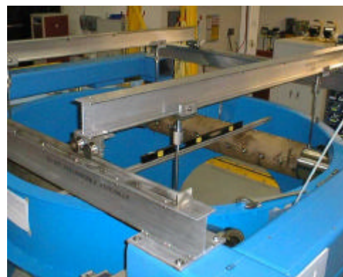
Figure 24. A Support Tube being Leveled. Figure 25. Both Support Tubes being Leveled.
