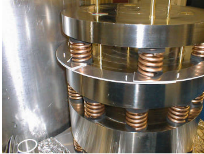
Figure 41. Spring Centering Jigs
