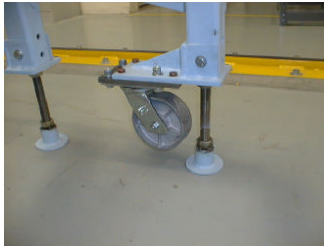
Figure 18. Roller System Foot Adjustment
