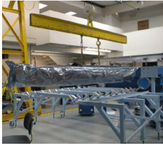
Figure 19. Support Tube Lowered on Roller System
