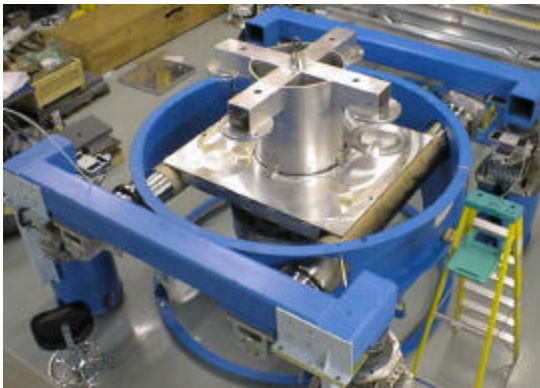
Figure 34. Support Table ready for Leg Stack Assembly
