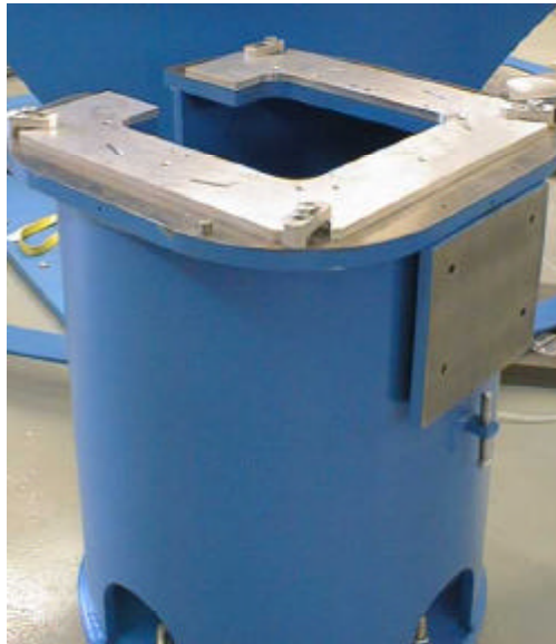
Figure 7. Adapter Plate Clamped in Place
