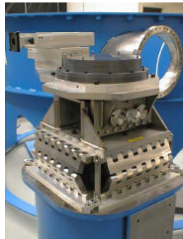
Figure 12. Air Bearing Base Surface on Mounting Plate
