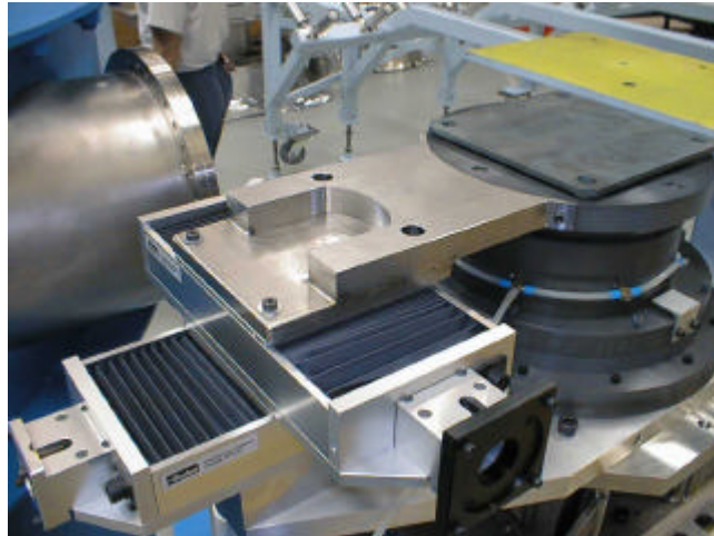
Figure 15. Air Bearing Mid Surface X-Y Positioning Jigs Figure 16. Flexural Pivot Jig Bolted in Position
