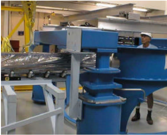
Figure 21. Support Tubes being Inserted into Chamber
