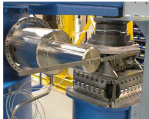
Figure 27. Support Tube being Clocked with Tool
