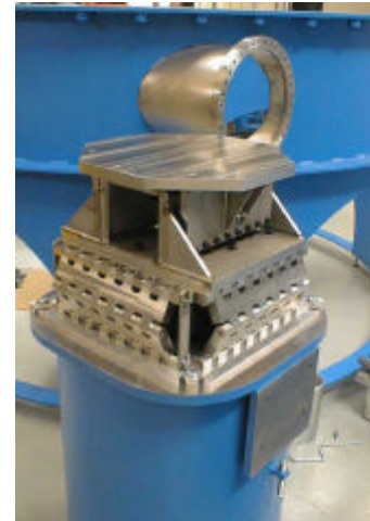
Figure 10. Fine Actuator Assembly Installed
