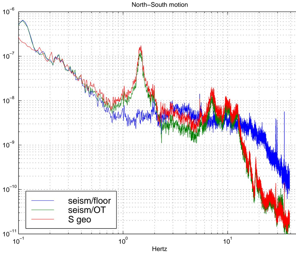
**Figure 8: Vibration isolation performance in v direction with real seismic input**
