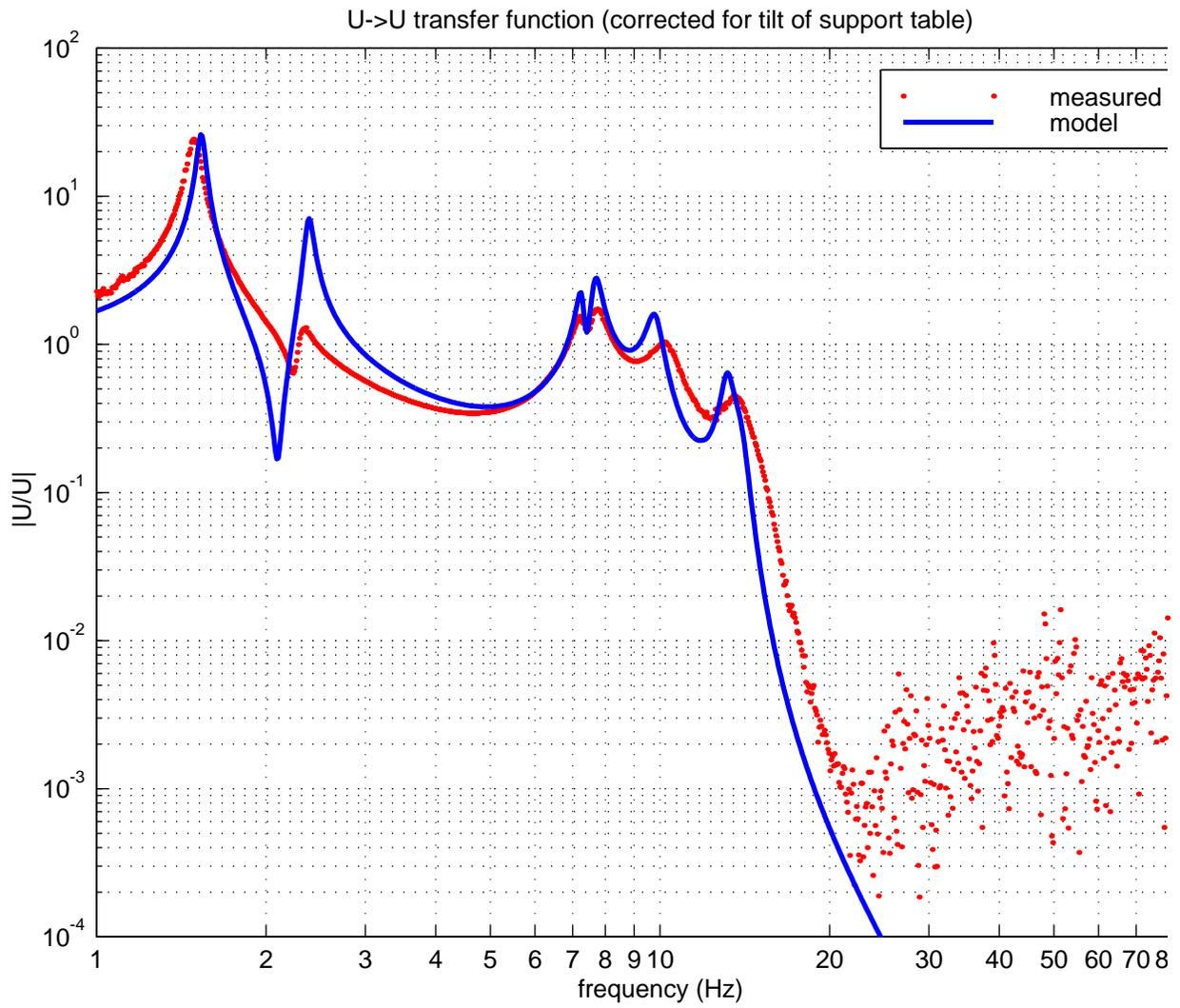
**Figure 4: Transverse horizontal transfer function**
