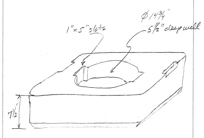
Circular cutaut has </8" diametrical play around the base of the carrier cover but x 11/2" rodial play around the top of the corrier conter)
