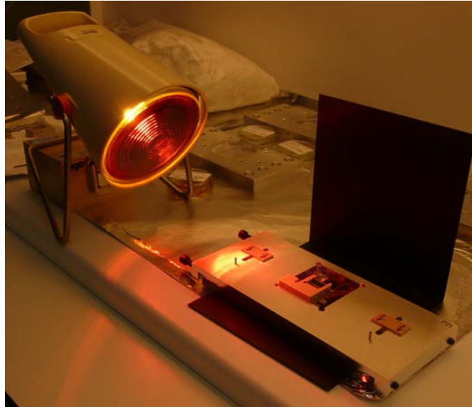
Figure 2.4 Heat lamp shining at glued prism
