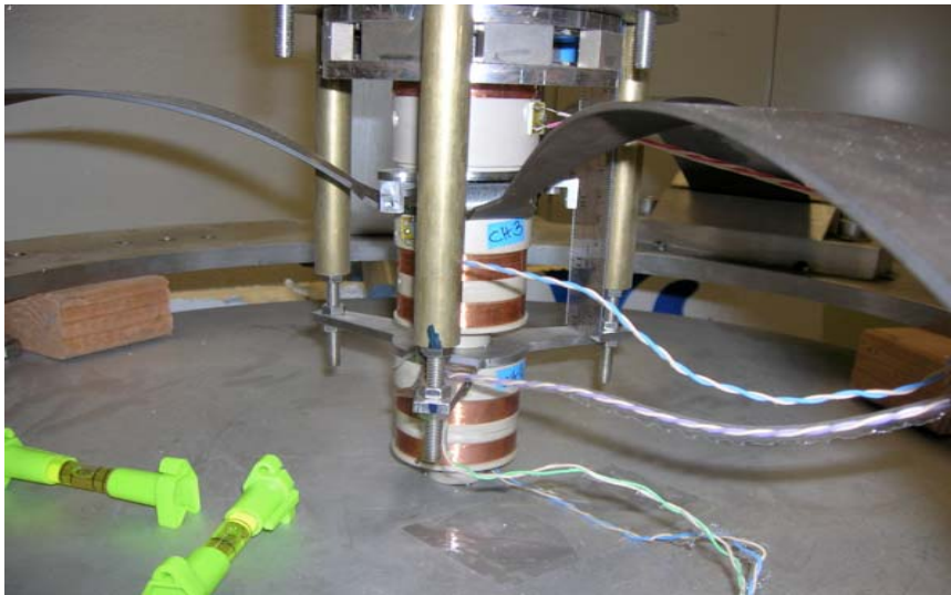
Fig.6:LVDTs on the GAS filter We want to work in the linear range of LVDT sensor and a calibration of this instrument is so necessary. To calibrate LVDT we added coins on the suspended load, acquiring at the same time both voltage (from LVDT) and height of the equilibrium point of the system.
