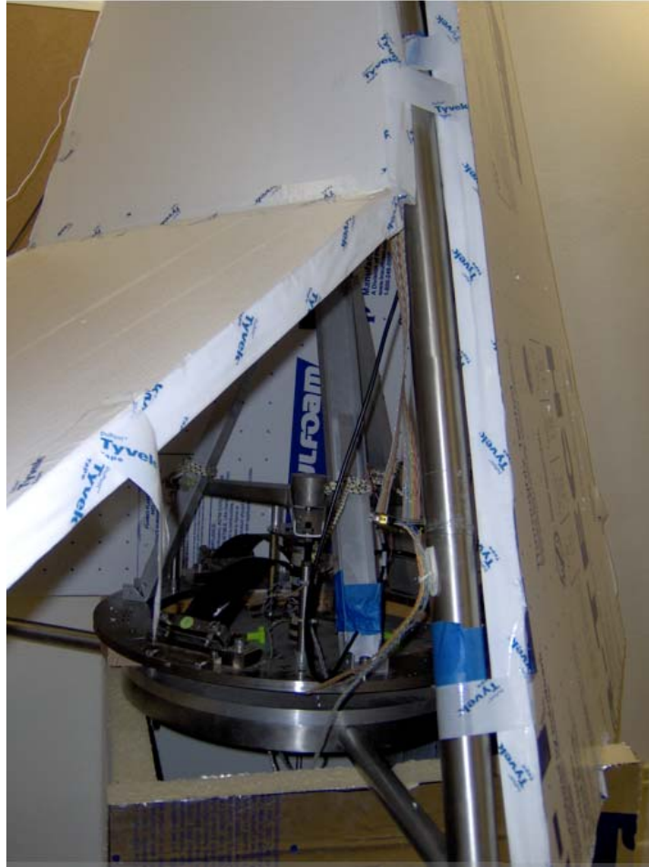
Fig.11: The box around GAS filter.
