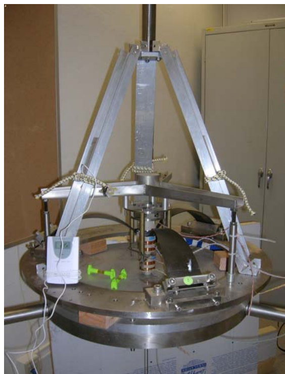
Fig.10:Actuator on the top of the GAS filter
