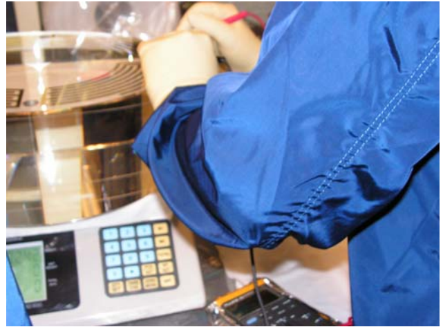
Figure 4.2 Measuring electrical resistance of the coating tracks
