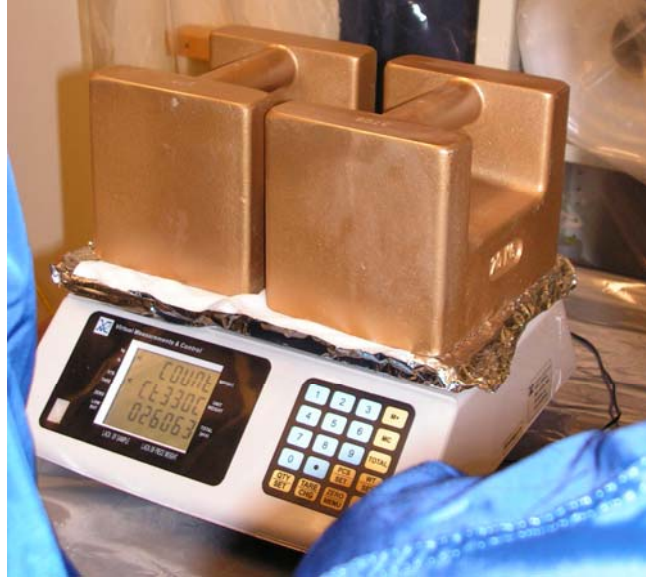
Figure 3.2 Weighing scale with calibration weights during calibration
