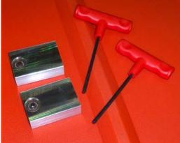
Carefully wipe clean the aluminum carrier with a dry clean room, lint free cloth. Take the aluminum mirror carrier to the processing area.
