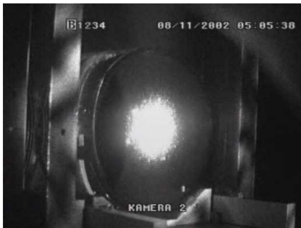
Figure 2: Image of the scattered light hitting on of the catchers at the far end. The intensity of the light on the catcher was estimated to be about 1.8 \text{ mW/cm}^2 . Overall 90 \text{ mW} of light are assumed to hit the front surface of the catcher.
