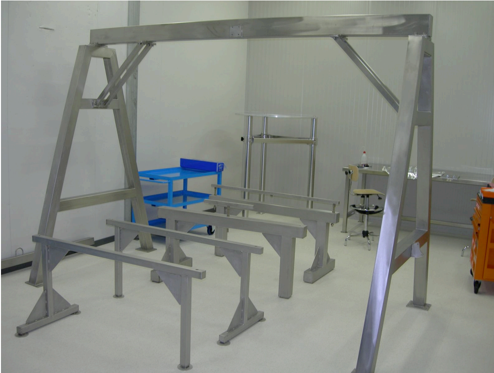
Clean-room-class A-frame crane, support and leveling horses and various tuning structures being readied in the clean room.
