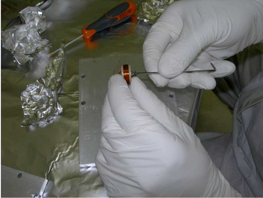
Primary coil being mounted on its plinth.
