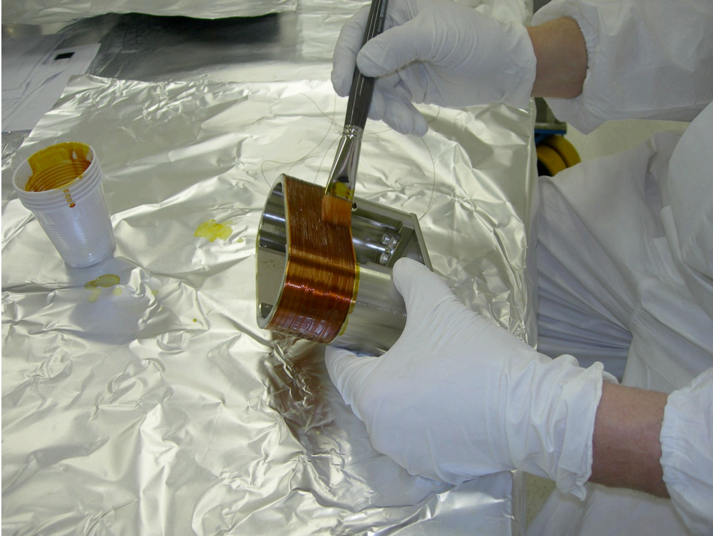
Voice coil actuators are coiled, then kapton painted and baked.
