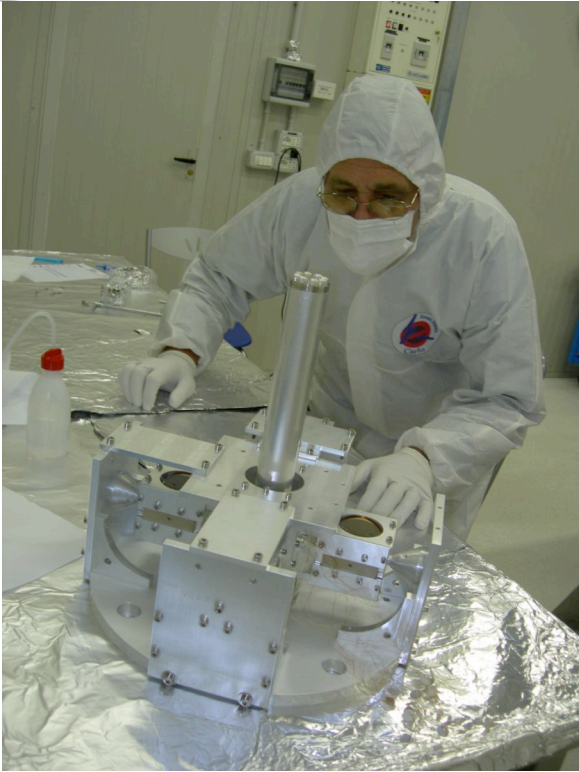
Roll Bar, controlling the table tilt stability, being mounted coaxial to the witness LVDT unit.
