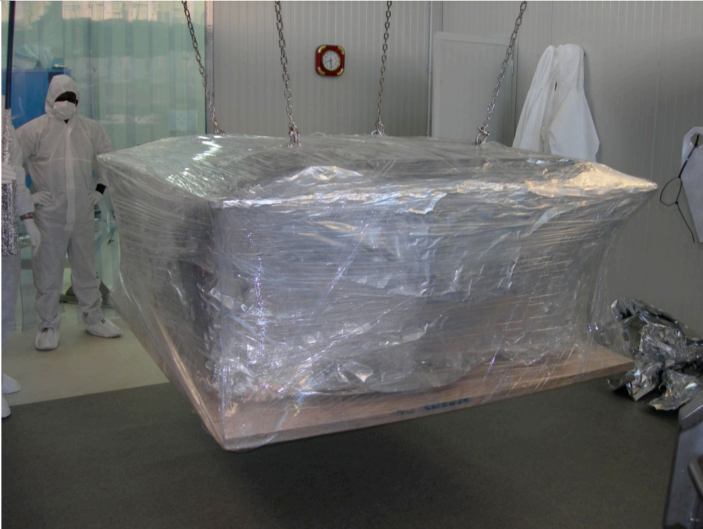
A final polyethylene wrapping precedes the assembly of the shipping crate.
