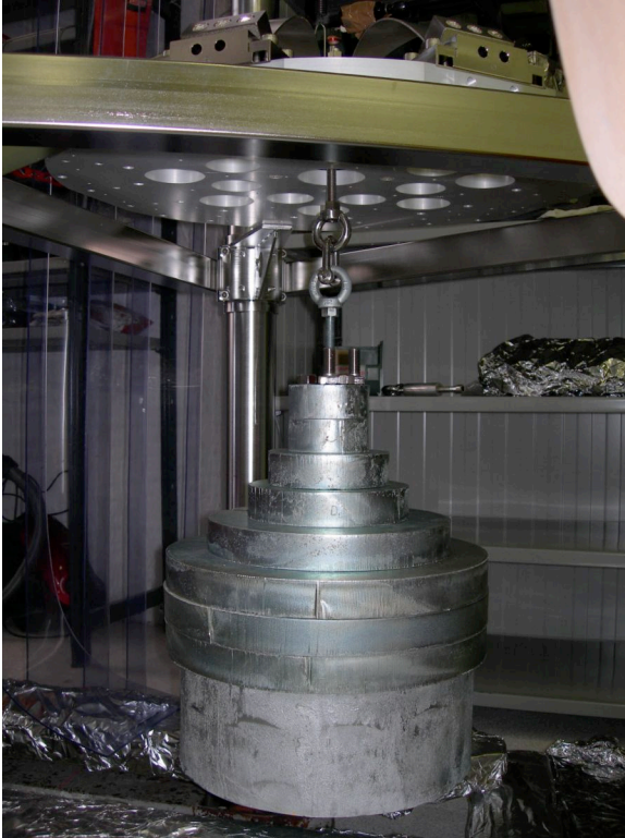
Each filter is loaded with 250 kg of clean mass for frequency calibration.
