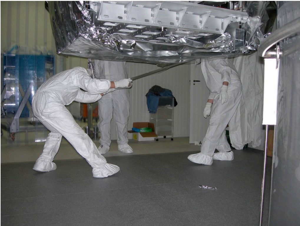
After bake-out the structure is wrapped in aluminum foil while still hanging below the oven cap.
