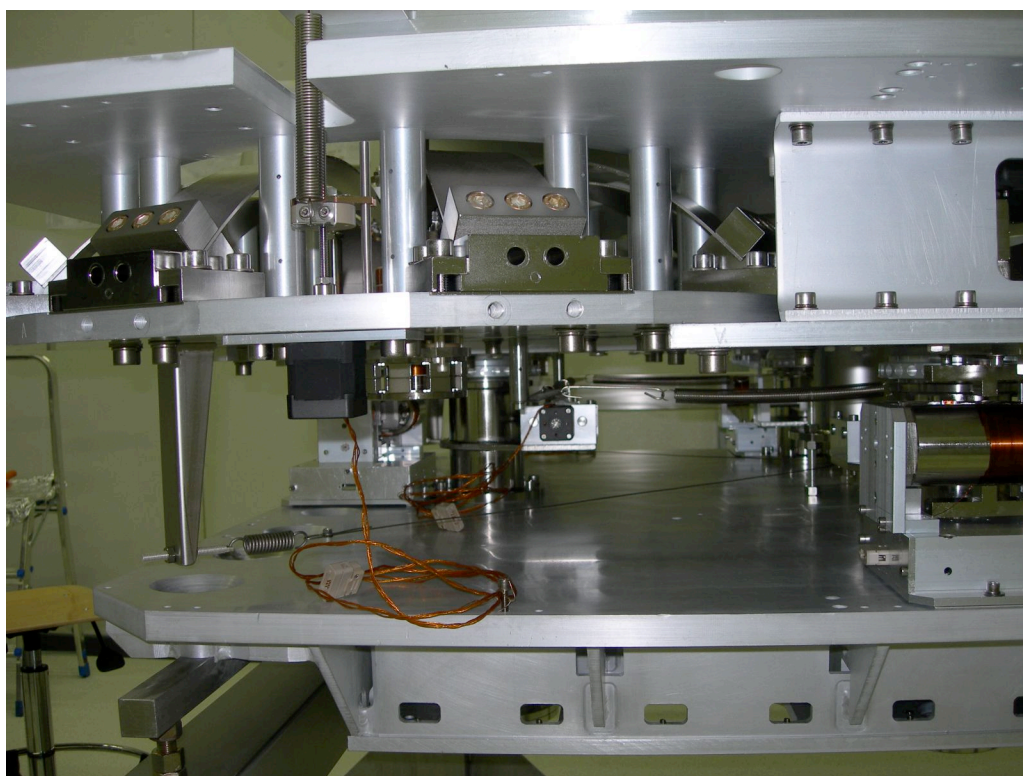
Finished assembly of the SAS structure, sensor actuator view. The horizontal tuning springs and the tilt control ones are visible in the background.
