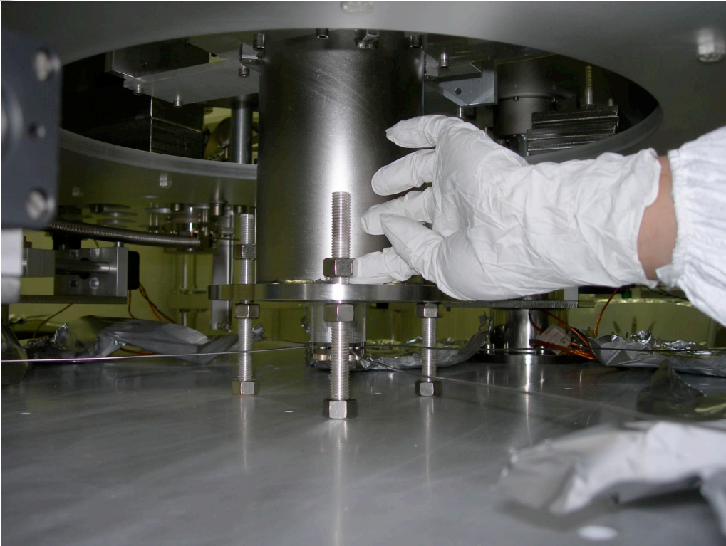
Witness LVDT being then fastened to the base structure. The double nuts provide vertical adjustment.
