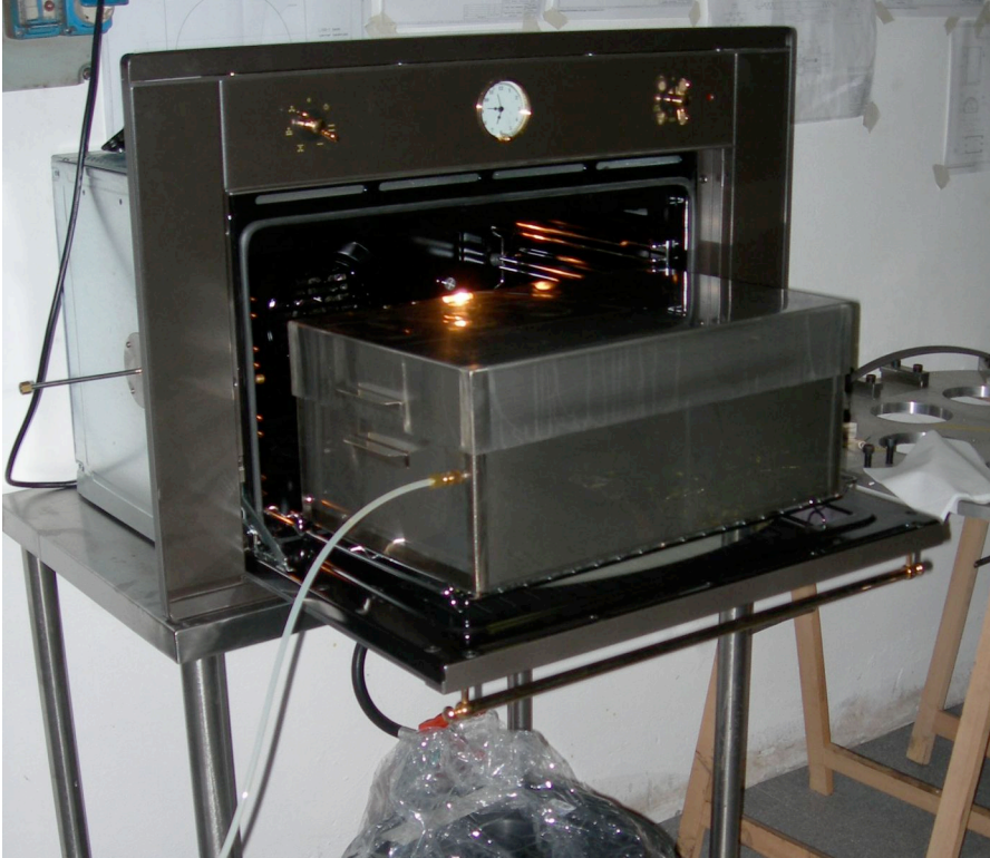
Small Bakeout Oven with its neutral atmosphere box (pre-purging)
