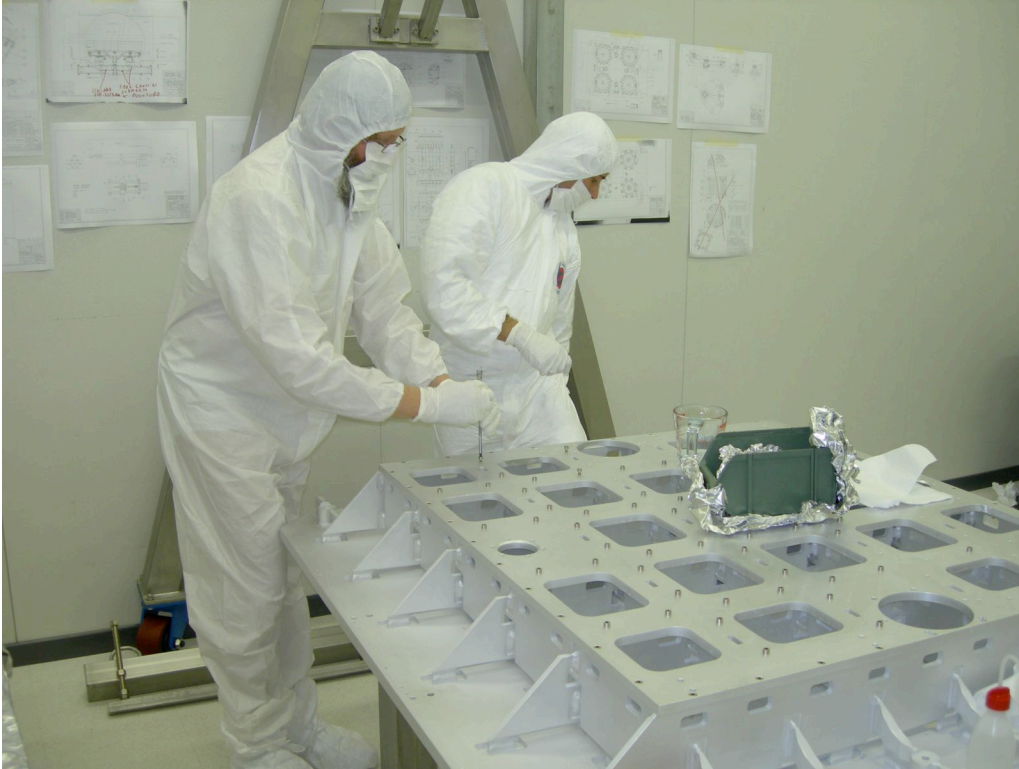
Base structure being assembled. It is composed of honeycomb weldment closed by a bolted bottom plate for cleanliness and machining precision. On the bottom right side is visible the shelf that will fit over the HAM cross pipes.
