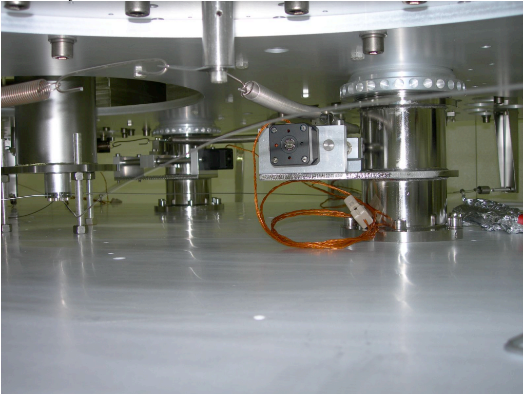
Witness LVDT being then fastened to the base structure. The double nuts provide vertical adjustment.
