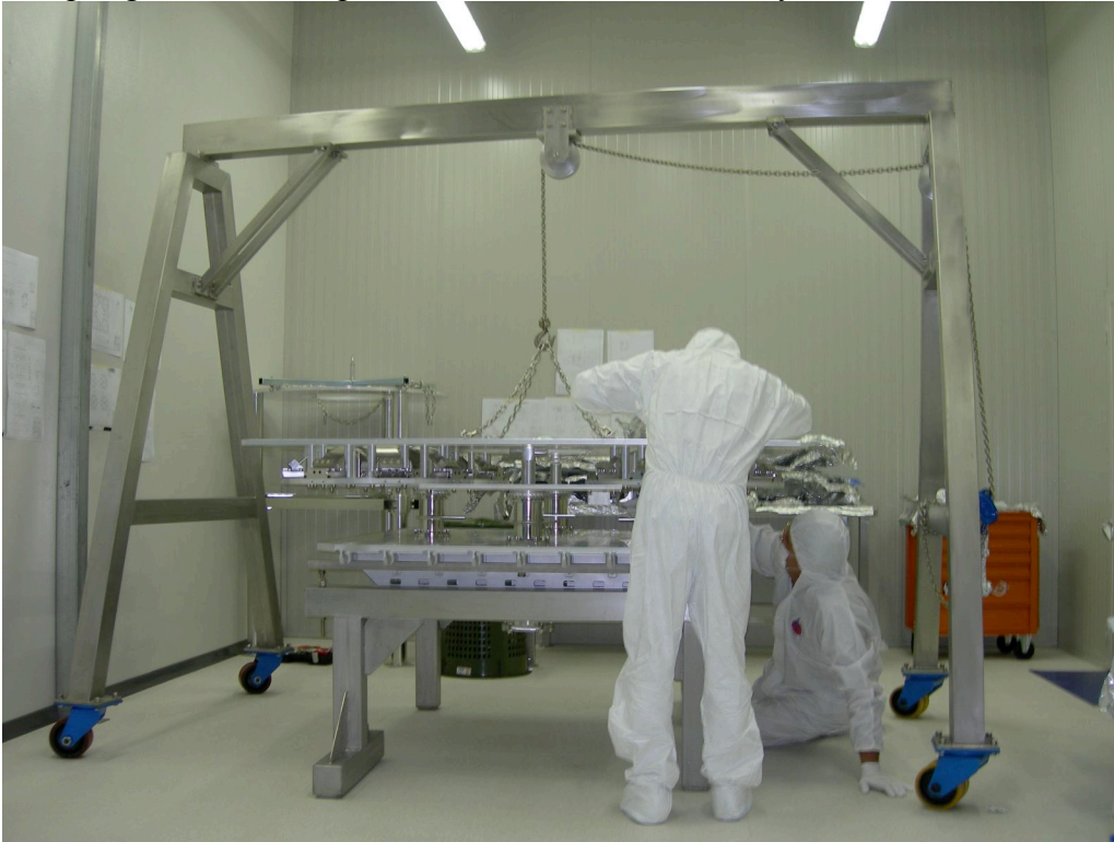
Positioning the spring box over the IP legs.
