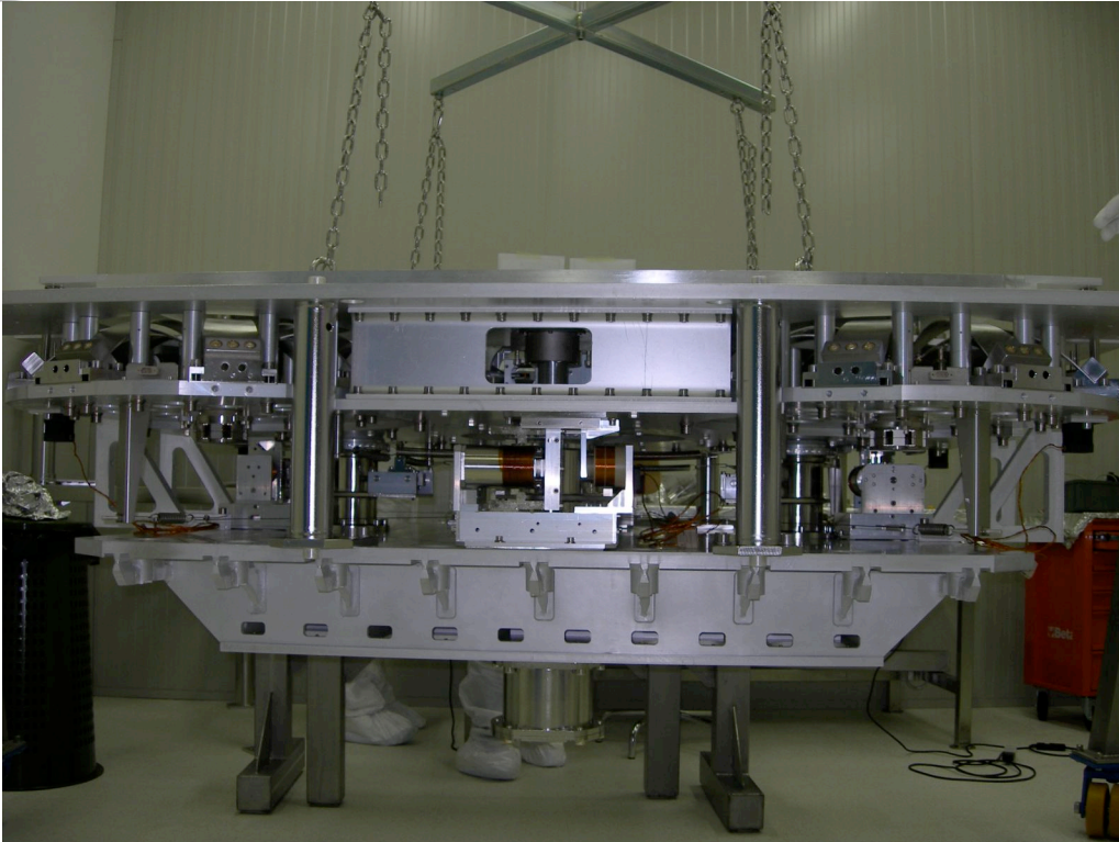
Transport tubes immobilizing the structure for transport.
