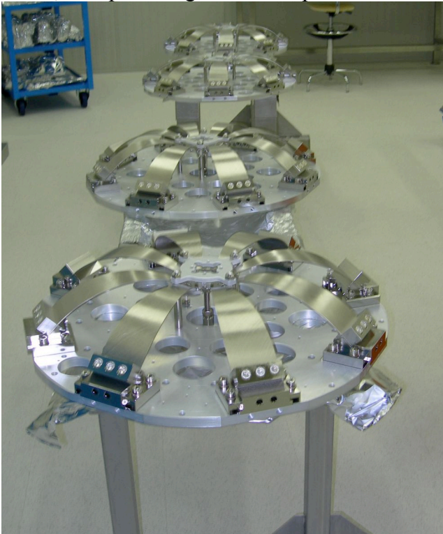
The four GAS Springs awaiting calibration and installation in the spring box.
