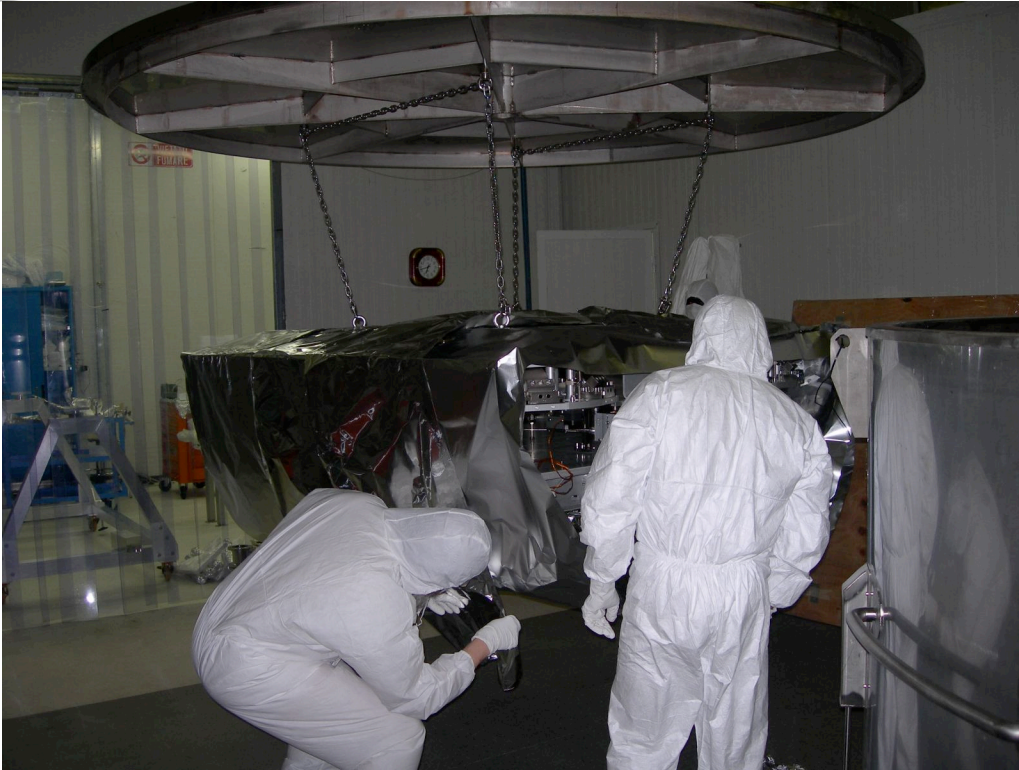
After bake-out the structure is wrapped in aluminum foil while still hanging below the oven cap.
