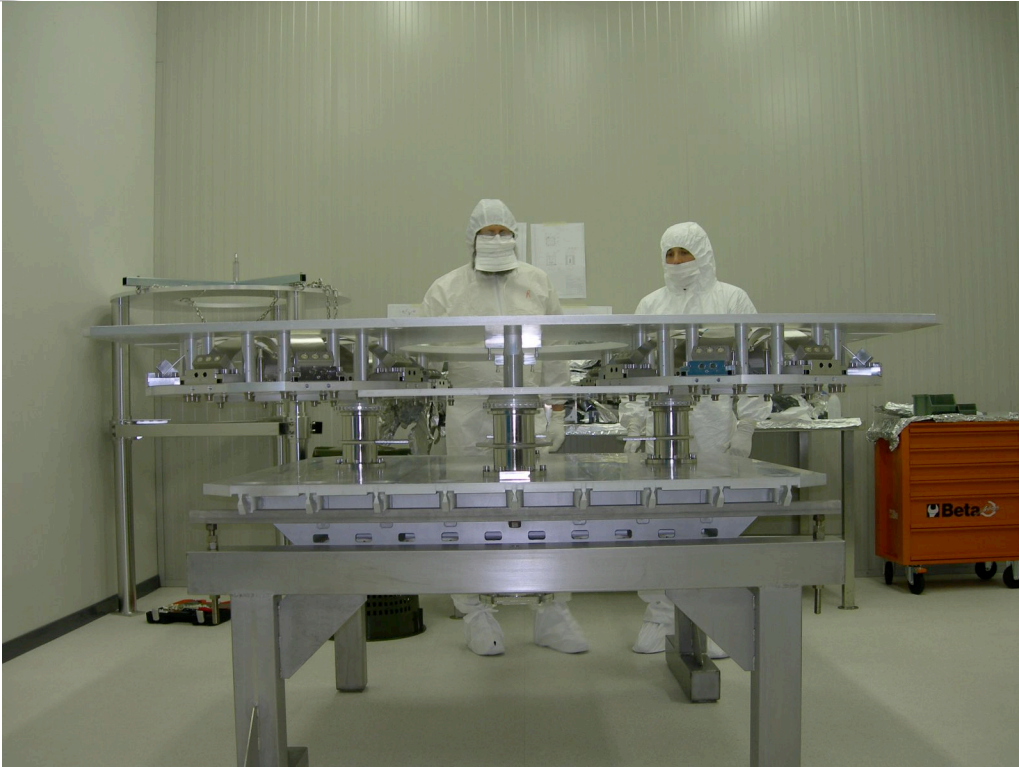
Finished, naked ,SAS structure, ready for instrumentation with LVDT sensors, Voice-Coil actuators and static positioning tuning motorized sleds.
