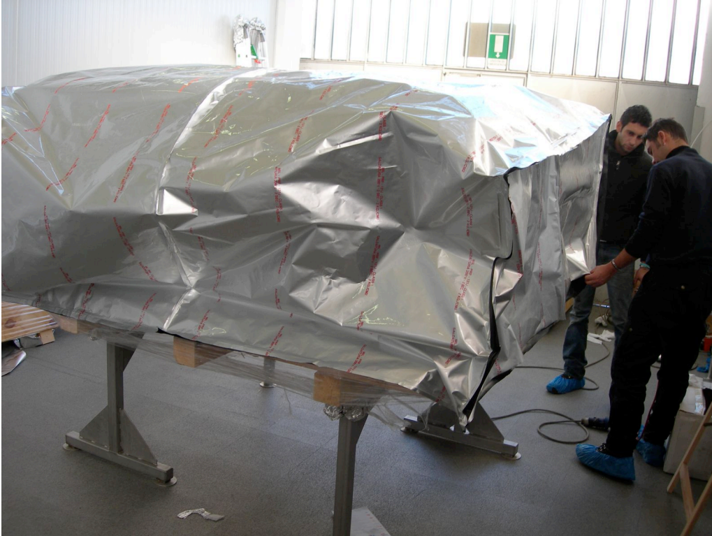
An air-tight weldable plastic film cap is welded to the base one, a window with a dust filter is applied on the bag to allow for air expansion during flight.
