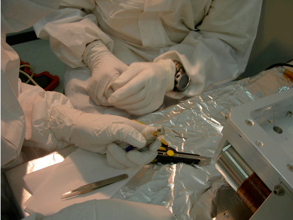
The LVDT voice-coil/actuator unit is cabled to its UHV connector.
