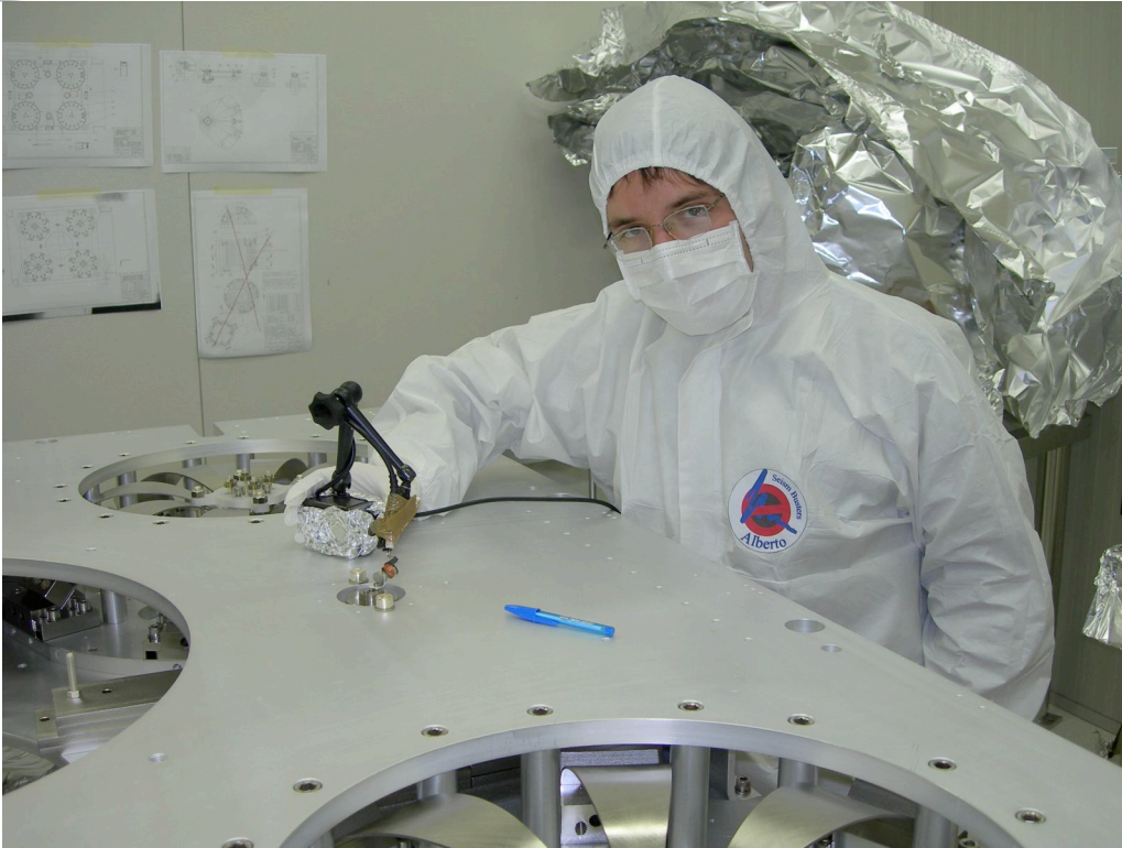
Testing the load sharing on the IP legs measuring the leg rigid body first resonance.
