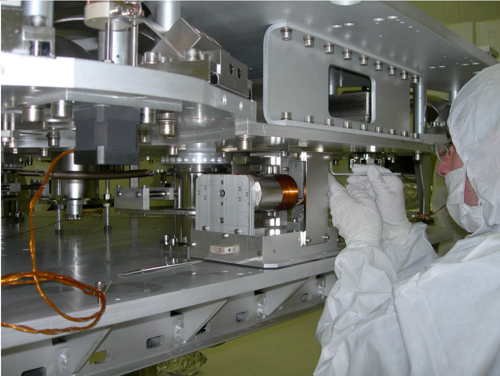
It is then installed between the base structure and the spring box.
