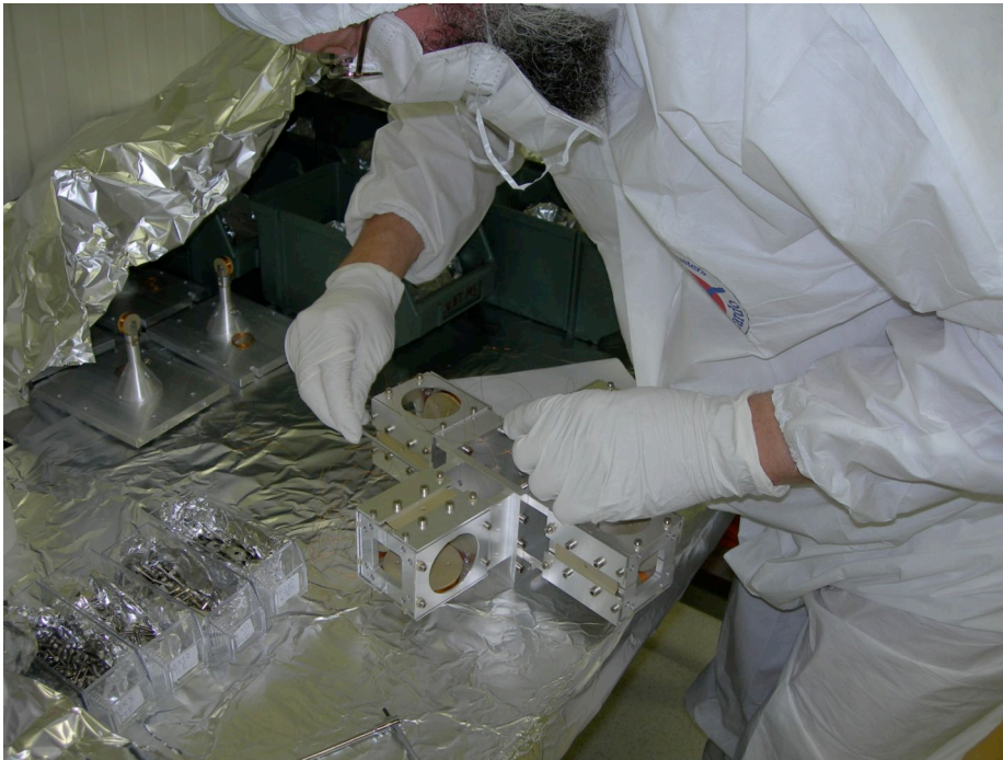
Primary coil being mounted on its plinth.
