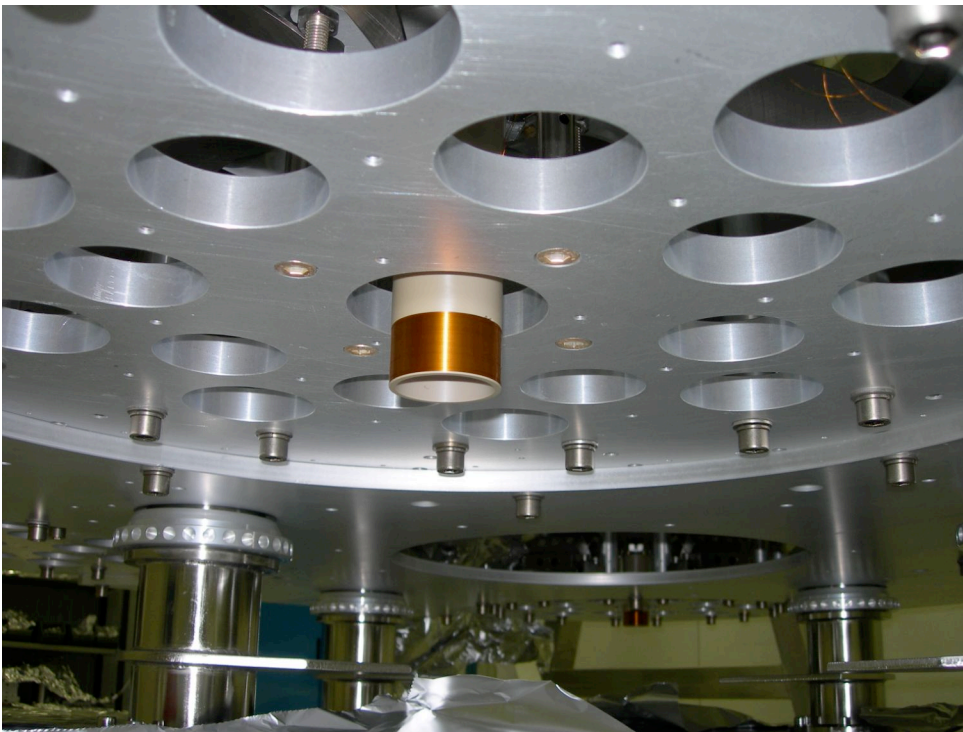
The LVDT primary and actuator coil cylinder is mounted on a GAS filter Key-stone .
