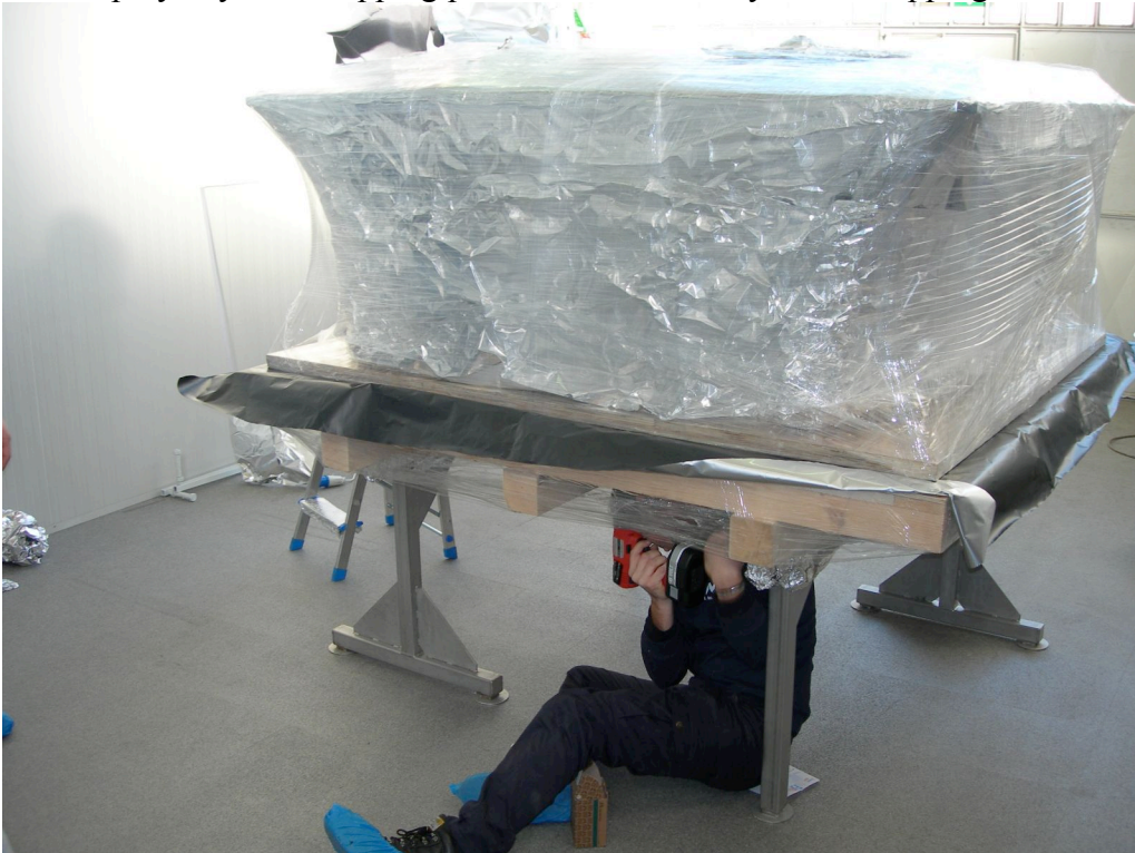
The crate bottom is screwed below the base plate, with a weldable plastic film imprisoned in between.
