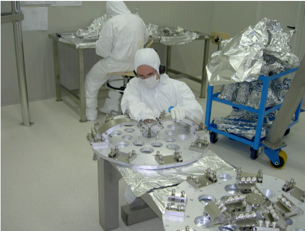
Clean GAS-Filter-blade pre-stressing tools. The SAS vertical attenuation is provided by a set of four Geometric Anti Spring (GAS) Filters
