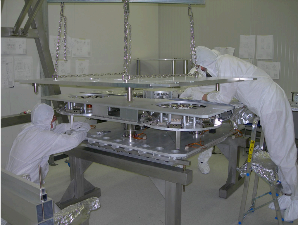
Optical table support plate being installed. It sits on a modified kinematic mount on the four filter key-stones. The optical bench slides over and bolts on this plate
