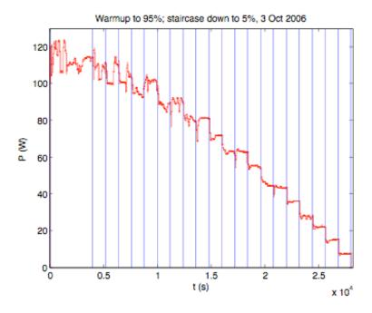
Figure 5: Effect of repeated negative step functions (nominally 5 W each, or approx 4.5% duty cycle)
