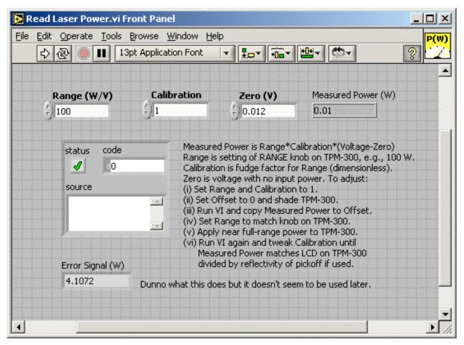
Figure 7: VI for reading laser power
