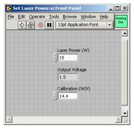
Figure 8: VI for setting laser power
