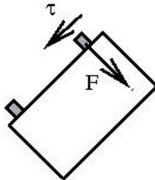
Figure 2: Forces created by the gradient in the magnetic field are assumed to act parallel to the dipole moment (worst case). Torques act perpendicular to the dipole moment.
