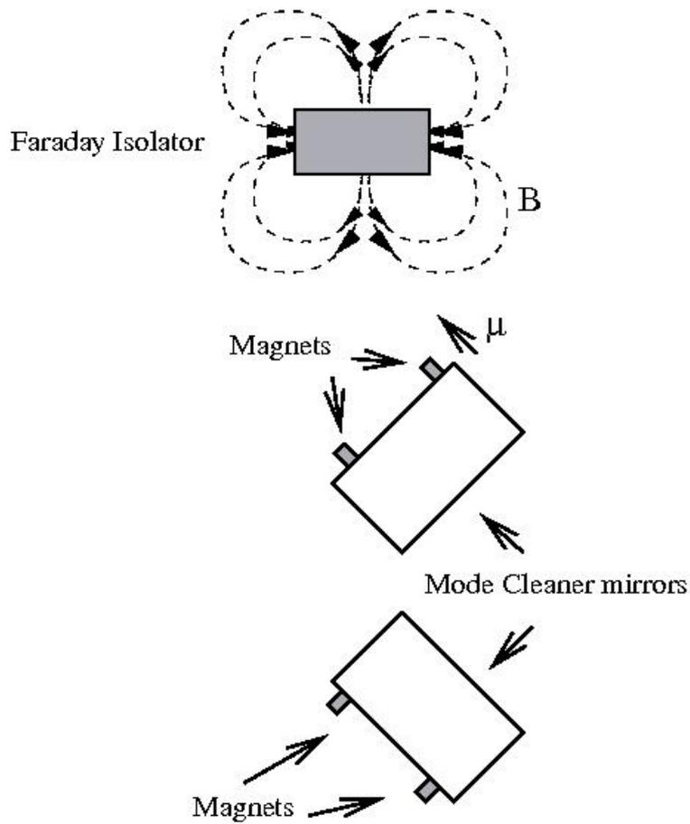
Figure 1: The drawing shows the two mode cleaner mirrors, the magnets, the isolator and the magnetic field lines. Note that this is just a sketch to describe the situation. The location of the isolator is not yet fixed nor is the shape of the conceptual magnetic field similar to the true magnetic field.
