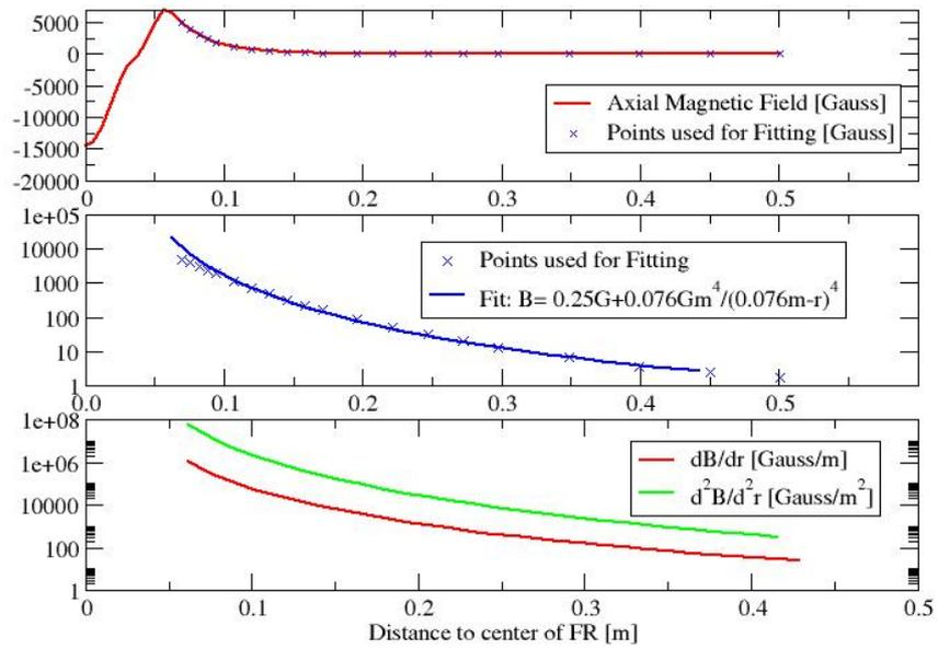
Figure 3: The axial magnetic field, a fit, and the first and second derivative.
