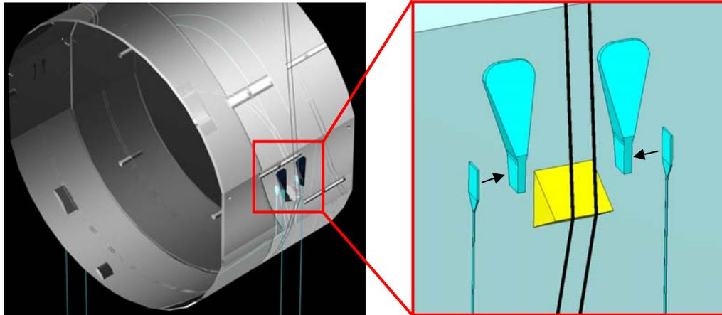
*Figure 4 Ears bonded to penultimate mass with ribbons welded in place. Note that the break-off prisms for the wire loops suspending the penultimate mass are also shown in this sketch.*
