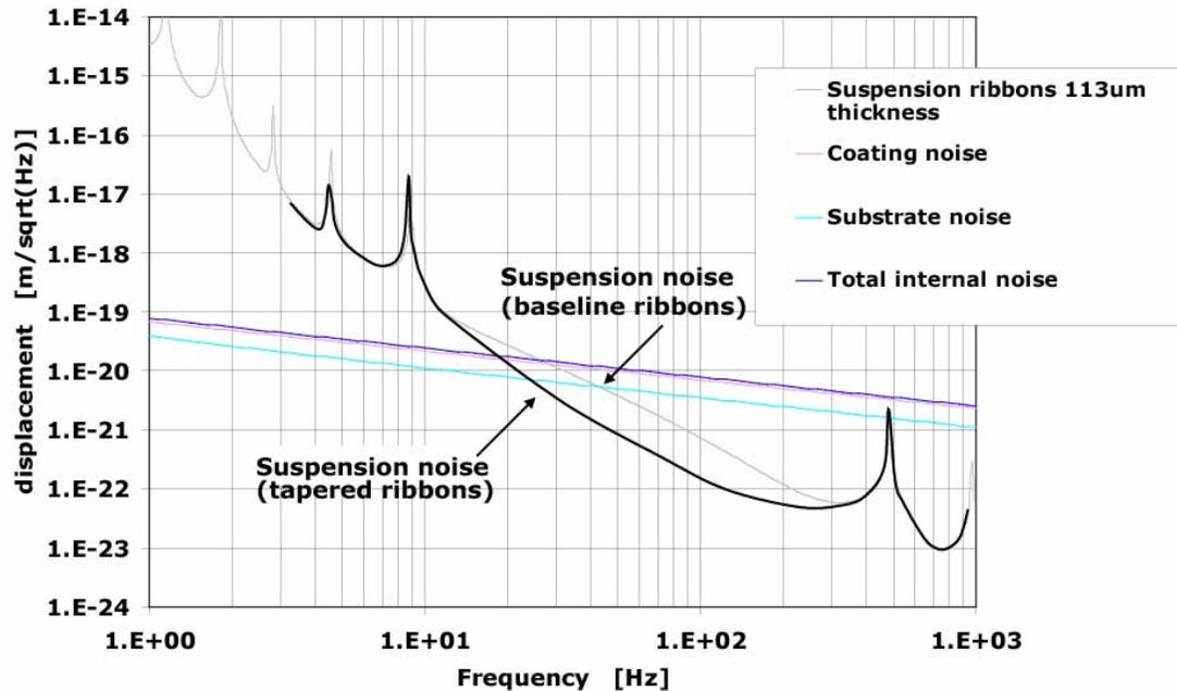
Figure 2 Suspension thermal noise curve and internal thermal noise curve for the coated 40 kg silica test mass. Note that thermal noise associated with the silicate bonded ears is not included.
