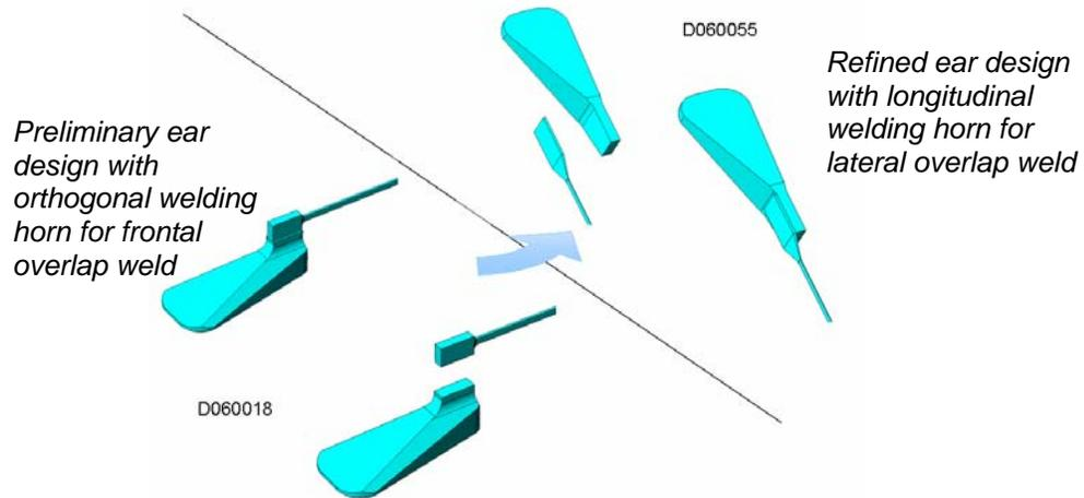
*Figure 3 Refinement of ear from design with orthogonal welding horn (D060018) to longitudinal welding horn (D060055). Ribbon modifications are discussed in Section 4.6.*
