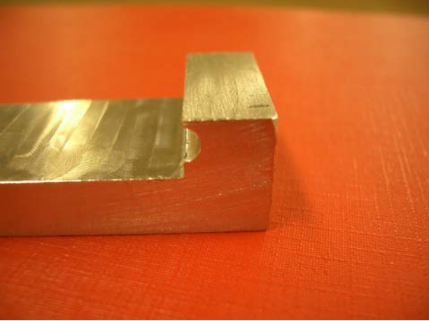
Figure 3 Loading hook with 1 mm loading edge
