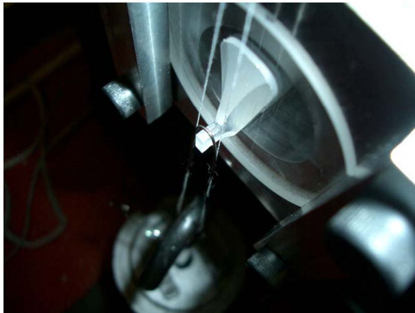
Figure 2 Load acting on bonded test ear on plane of the proposed ribbon weld to produce correct moment
