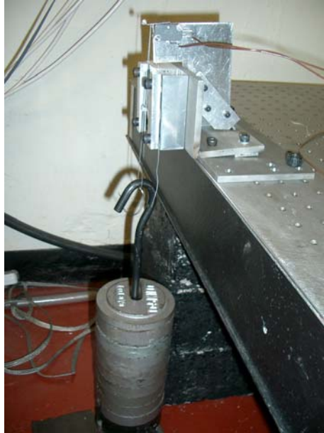
Figure 2 View showing 12 kg load on bonded ear
