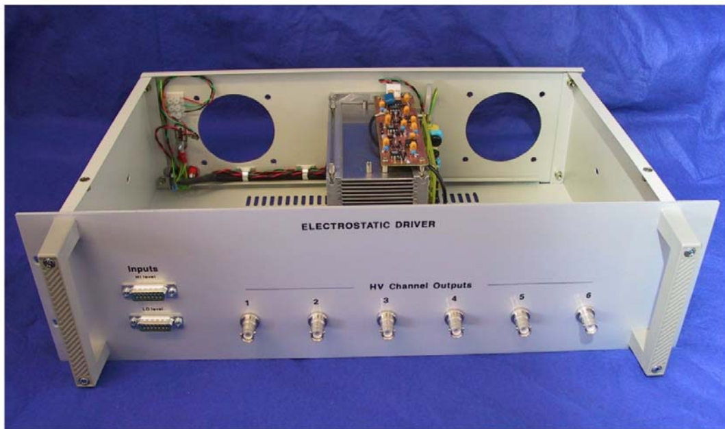
Figure 2. The prototype ESD amplifier showing the Analog PCB mounted on top of the slotted-heatsink, and one HV PCB mounted on its RH side (two HV PCBs were ultimately mounted on the heatsink).
