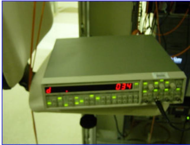
Figure 2. Clock Fanout Board's Output Jitter as Measured by the SR620
