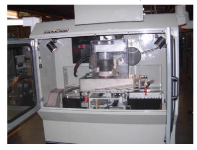
Fig.6 Internal view of the machine. A polycarbonate transparent box (for high voltage safety) hosts the rotating ultrasonic head with the centering slides and the piezoelectric transducer cooling system. The working table is surrounded by the antisplash container and by the secondary high-flow slurry feeding. Below the table (the protection carter has been removed) is visible the load control system.
