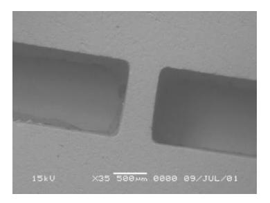
Fig.4 SEM micrograph of a 400 µm thick flex-joint machined from a 3-mm thick sapphire single crystal wafer.
