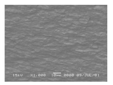
Fig.3 SEM micrograph of a single crystal sapphire surface machined in our laboratory with boron carbide 220 mesh. Irregularities of 1-5  $\mu$ m can be observed.
