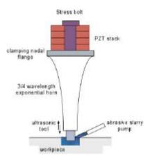
Fig.2 Ultrasonic machine tool schematic
