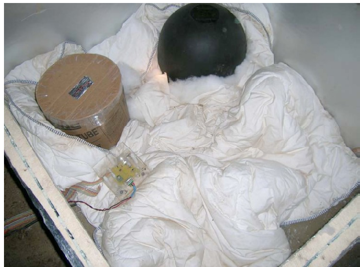
Figure 4: A Trillium T-240 at the 2000ft level surrounded by the thermal acoustic box to isolate it from its surroundings [1].
