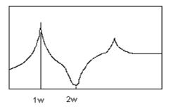
A resonance should be present at the operating frequency of the diode  $(1\omega)$ , and a notch should be present at twice the operating frequency  $(2\omega)$ . The second peak is not required, and is a secondary characteristic of the circuit.
