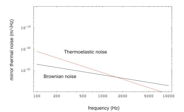
Figure 4: Expected noise in LIGO with sapphire mirrors and unchanged spot size. Thermoelastic noise is not nearly so much of a problem as in Braginsky's plots, because he underestimated our spot size.
