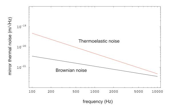
Figure 6: Expected noise in the proposed 40-meter with sapphire mirrors. Thermoelastic noise still dominates, but it is closer to LIGO's expected value.
