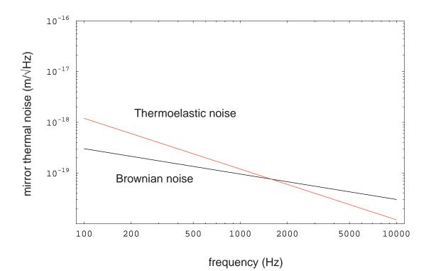
Figure 2: Expected noise in the TNI with fused silica mirrors. Note the change in scale relative to Figure 4. The crossover between noise sources around one kilo-Hertz would be very interesting to observe.
