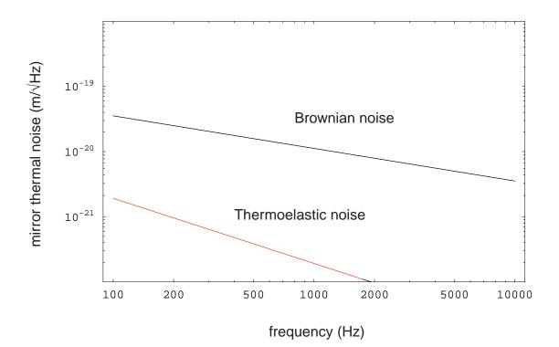
Figure 3: Expected noise in the proposed 40-meter with fused silica mirrors. This should closely mimic LIGO's thermal noise curve. Note that this scale is the same as that of Figure 4.
