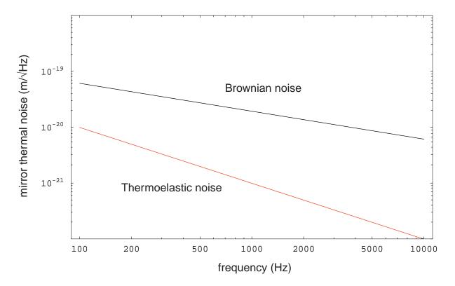
Figure 7: Could the old 40-meter have seen thermoelastic noise? Not likely, if its g-factor were 1/3 as is LIGO's. Brownian noise would still have been dominant.
