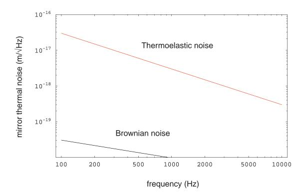
Figure 5: Expected noise in the TNI with sapphire mirrors. Thermoelastic noise is huge. This should provide an initial confirmation of Braginsky's thermoelastic noise prediction.
